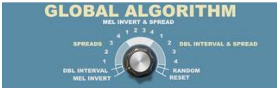
The Global Algorithm is how you change the algorithm when in Global Mode. Of course, you can use this as an on the fly controller for the whole device, but another great usage for it is to help you fine tune the individual algorithms, particularly the Spreads – then once this is done you can go to town with the Randomizer on the Sequencer.
