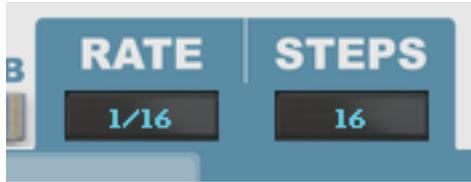
These controllers are only applicable to the Sequencer Mode. The Rate controller specifies how often the step will change when the sequencer is running, and it has the following values available:
