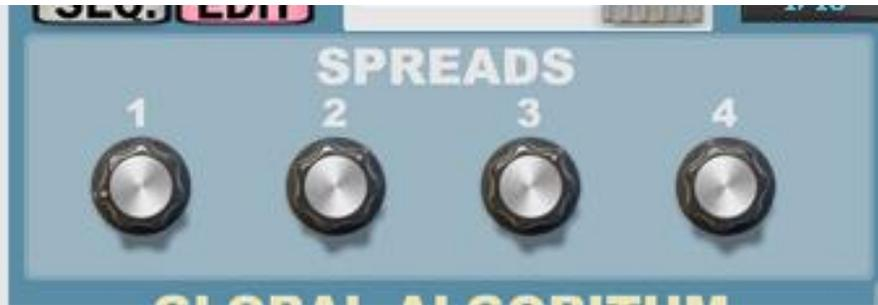
There are 4 Spread controls in the Edit Panel. Each of them ranges from 0-12, where 0 is effectively off and 12 is a full octave. Each value simply adds or subtracts the appropriate amount to the incoming notes, depending on which Algorithm is selected.
