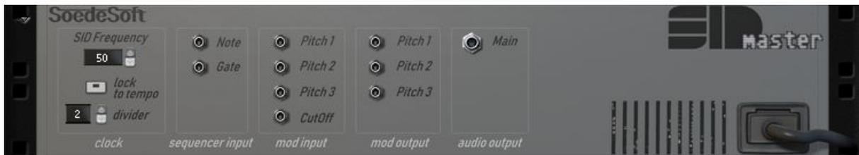
The SIDmaster operates at a base frequency of 50 Hz, but can be modified e.g. to 60 Hz (which for example is the case in the USA).
